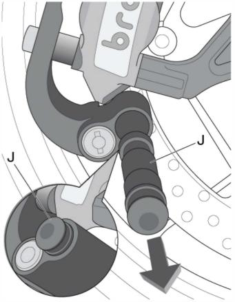
7. Insert the pin (I) into the hole where the black plug was removed. The key must remain rotated fully in the unlocked position to allow the pin to be inserted. While the pin is fully inserted being held by finger pressure, the key can be rotated anti-clockwise and removed. The cylinder uses a dead-bolt latch to hold the pin in the lock body.
